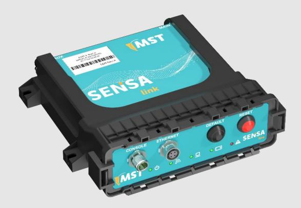
Reliable, fast roaming wireless connectivity for mobile mining equipment.
