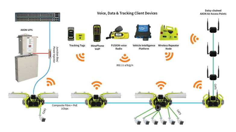
AXON infrastructure - A platform designed for supporting the many devices and applications required in the digital mine.
