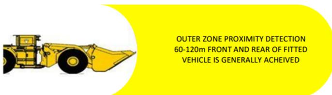
**Figure 1: MST's Proximity Detection Outer Zone**
