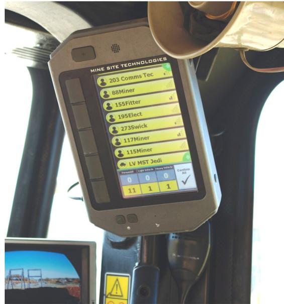
Figure 3: MST's Proximity Touch Screen inside a vehicle cab
