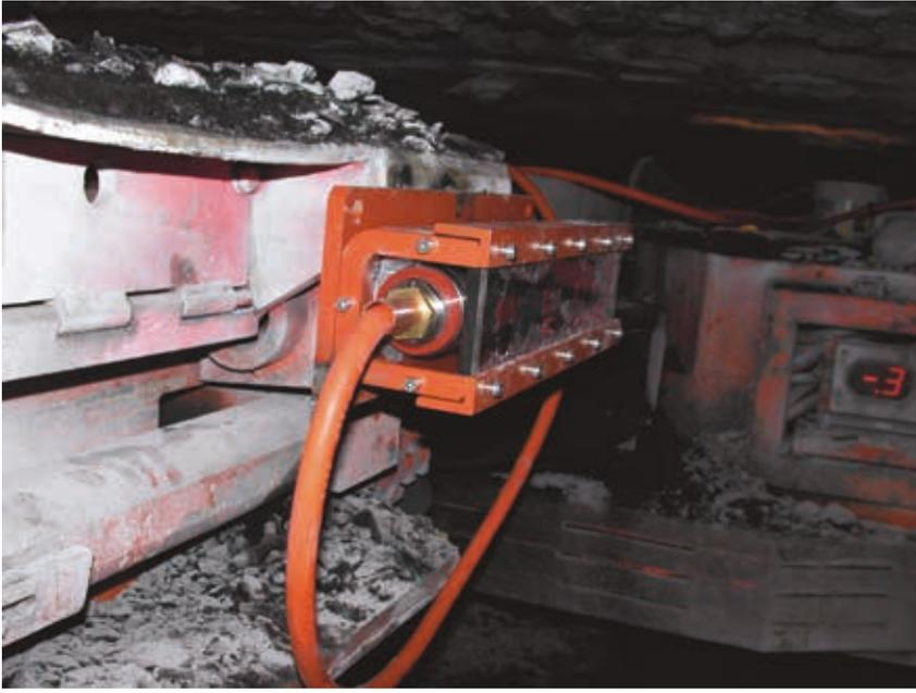
The proximity detection system uses a magnetic field generator mounted on a shuttle car.
