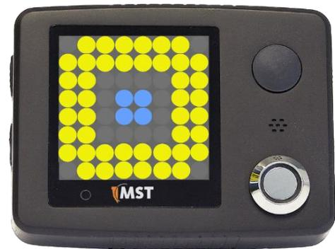
The 100mm x 135mm **display panel** with 8x8-tricolour LED array provides audible and visual alarms to the machine operator. A push-button allows the operator to suppress the alarm, which reactivates after a programmable time-out.
