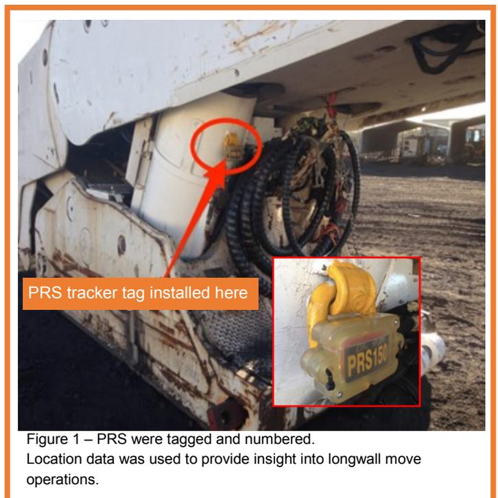
Figure 1 – PRS were tagged and numbered. Location data was used to provide insight into longwall move operations.
